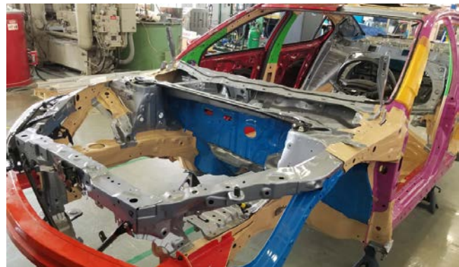
COSI powder coated the frame of the car in different colors to show the different materials used.
